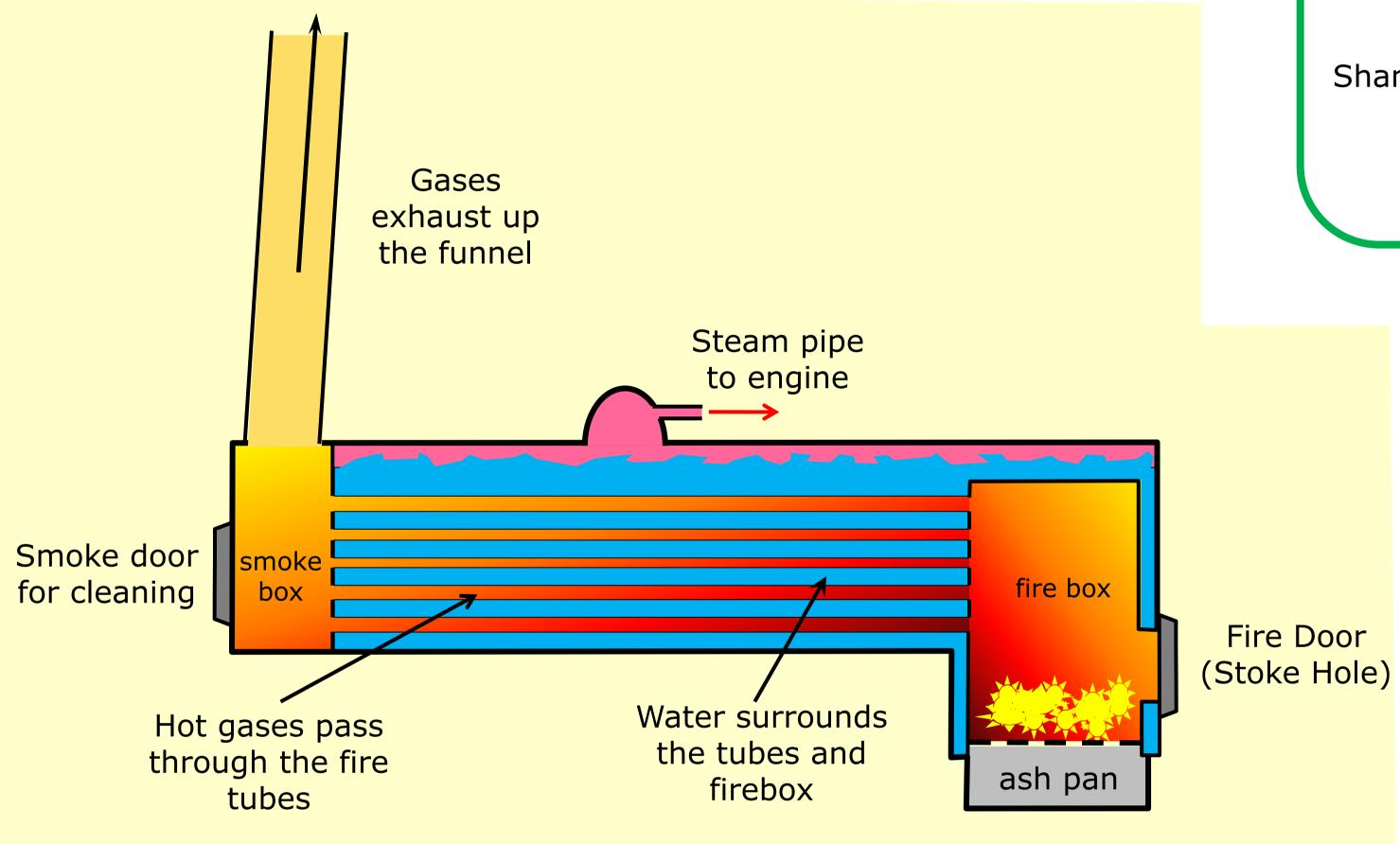
The Stoke Hole is at the back for a Locomotive boiler, or at one side for a Launch boiler.
