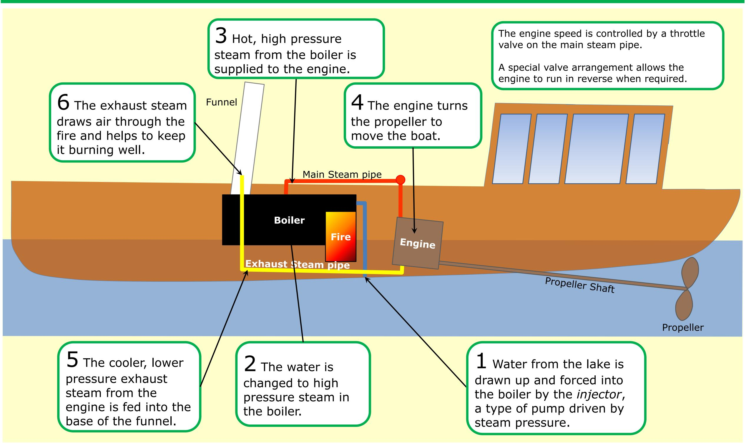
When the exhaust steam is fed into the funnel, it produces the characteristic puffing sound associated with steam locomotives. This is less pronounced on Shamrock, because a silencer is fitted.
