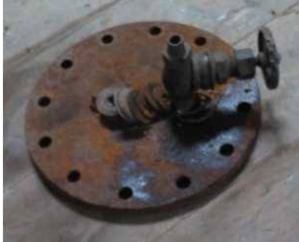
Figure C-5: Steam Dome Blanking Flange
