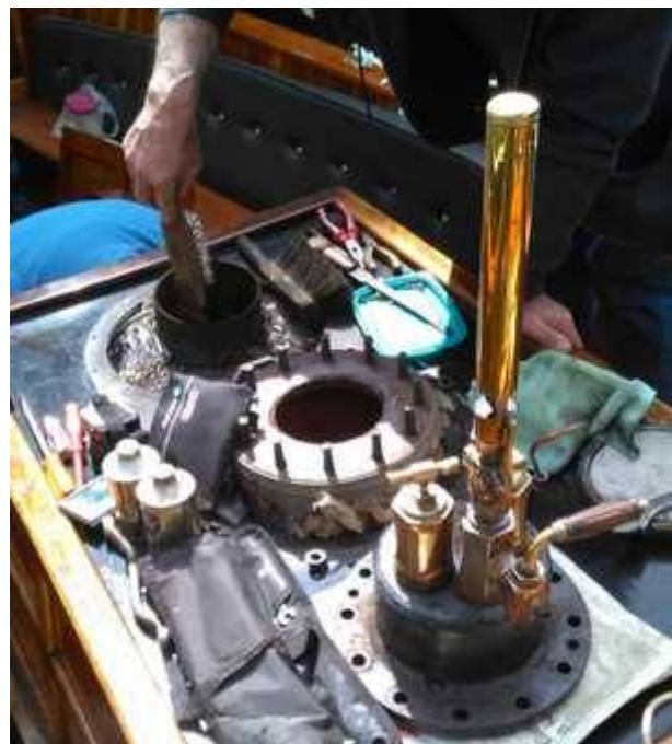
Figure C-4: Cleaning the Uptake
