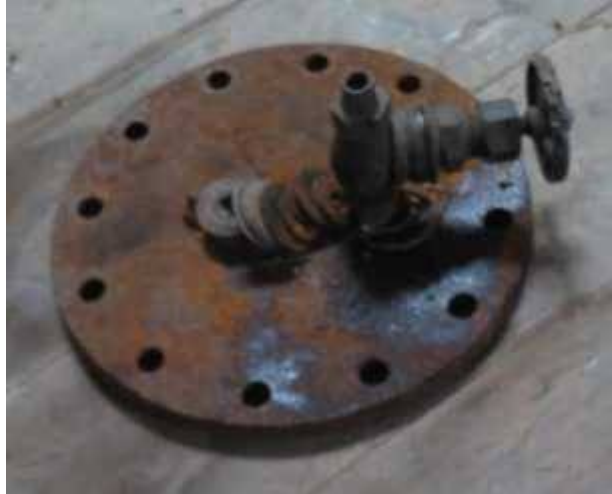
Figure C-5: Steam Dome Blanking Flange
