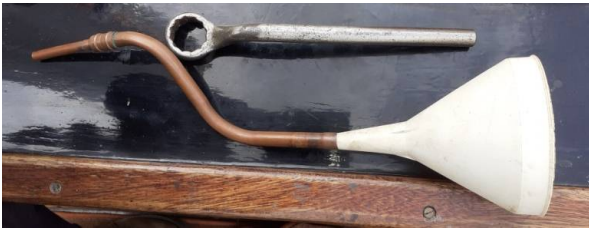
Figure 4-2: Cranked Funnel and Spanner
