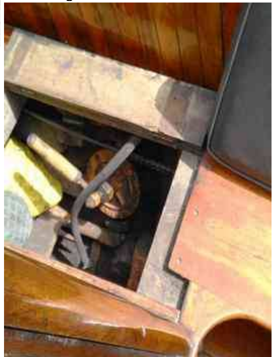
Figure 4-11: Hand Bilge Pump
